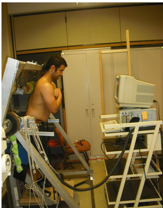
Figure 10. Visual feedback provided by monitor helps to control the required extension force.
