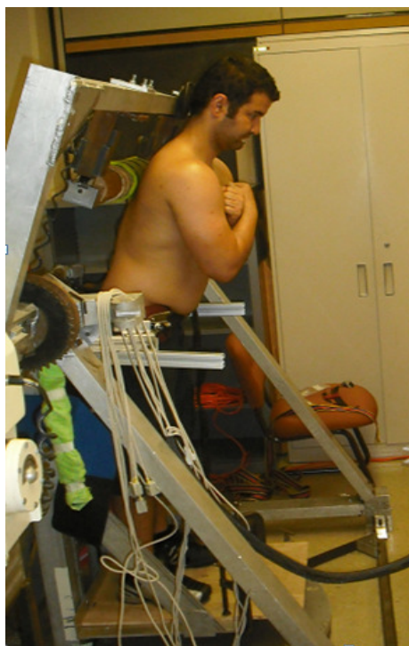
Figure 8. Asymmetric reference frame: Maximal extension of the trunk against a stationary surface.
