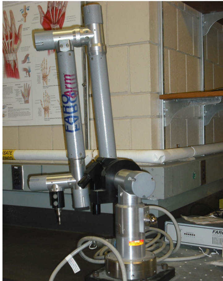
Figure 26. FARO Arm is a portable 3D/6D digitizer.
